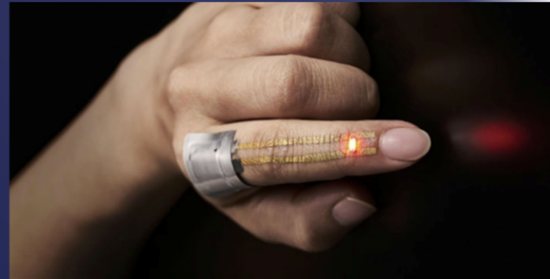
The electric current from a flexible battery placed near the knuckle flows through the conductor and powers the LED just below the fingernail. All images courtesy of Someya Laboratory.
